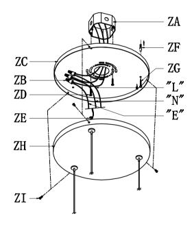
Black wire from ceiling(junction box) attaches to "L"wire from the fixture.
