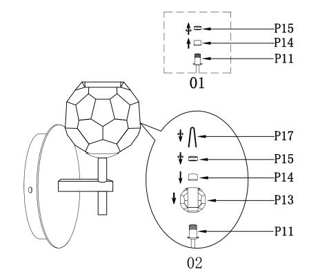
01. Unscrew the lamp holder ring (P15) counterclockwise, and then remove the iron tube (P14); 02. Put the crystal lampshade (P13) on the lamp cup (P11), hold it by hand, and then put it into the iron tube (P14), Then fix it to the lamp cup (P11) with the lamp ring (P15), and finally tighten it with a "U" wrench (P17).
