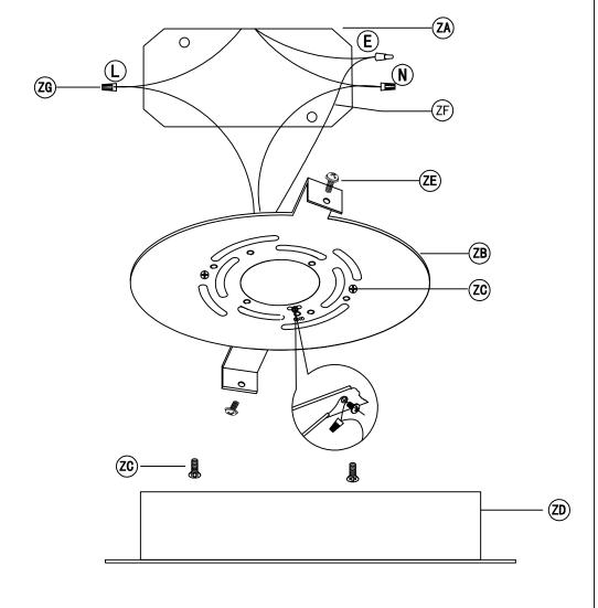
IMPORTANT: Test sockets with bulb before dressing the fixture.
