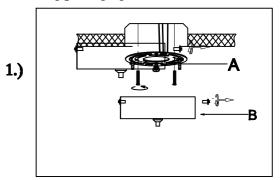
Step 1: Remove mounting bracket (A) from canopy (B) and install to electrical box.
