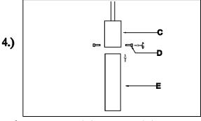
Step 4: Insert glass (E) into cup (C) and secure using screws (D) provided.
