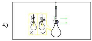
Step.4: Install G9 bulb (E) provided. Gently turn glass (F) onto socket (D) to secure.
