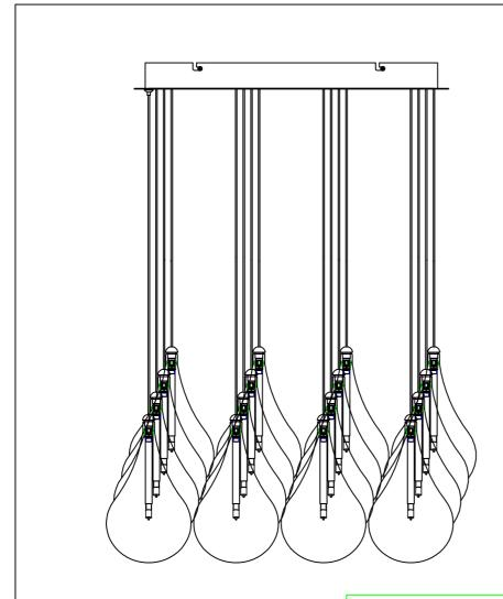
WARNING: Wires need to be connected to transformer found in canopy and should not be connected directly to power source or a short may occur
