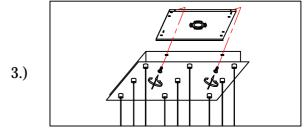
Step.3: Tighten screws (D) on the sides of the canopy (C) to secure the fixture.
