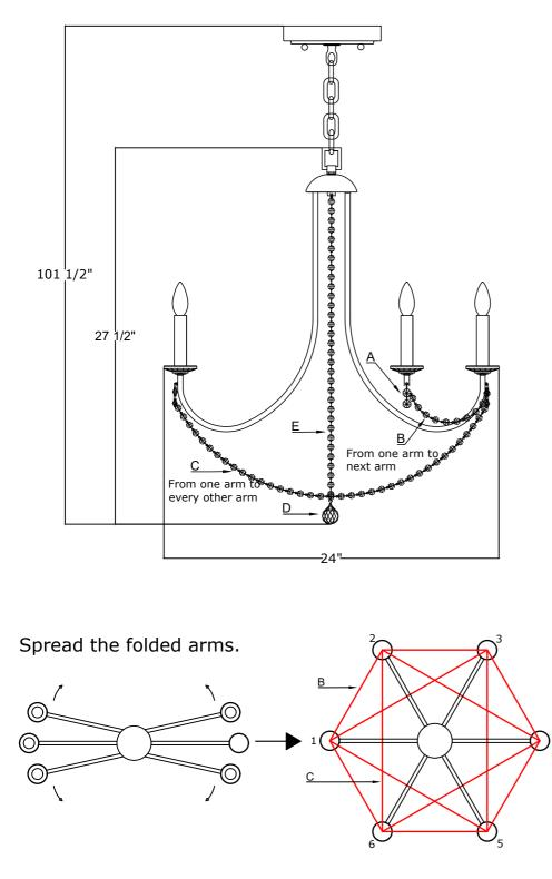
WARNING: Electrical Danger Turn Power Off All electrical components must be installed by a licensed electrician in accordance with the National Electric Code and the appropriate local electrical codes. LISTED Vou will need 6- Candelabra Base Bulb 40 Watts recommended 60 Watts Max. USE LED BULBS FOR EXTENDED USE
