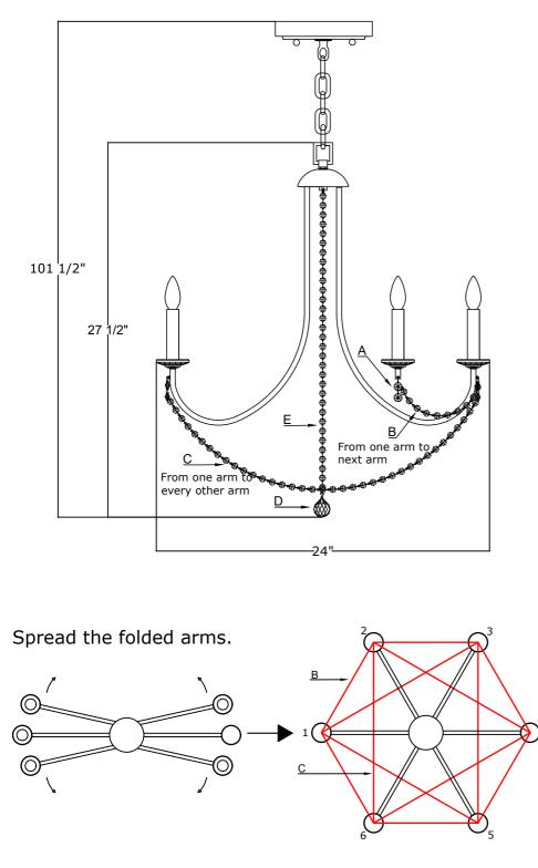
WARNING: Electrical Danger Turn Power Off All electrical components must be installed by a licensed electrician in accordance with the National Electric Code and the appropriate local electrical codes  $\mathcal{M}$ You will need 6- Candelabra Base Bulb 40 Watts recommended 60 Watts Max. USE LED BULBS FOR EXTENDED USE The fixture is Dry rated **HOW TO INSTALL:** Place the fixture parts on a soft cloth-covered platform before installation of fixture.
