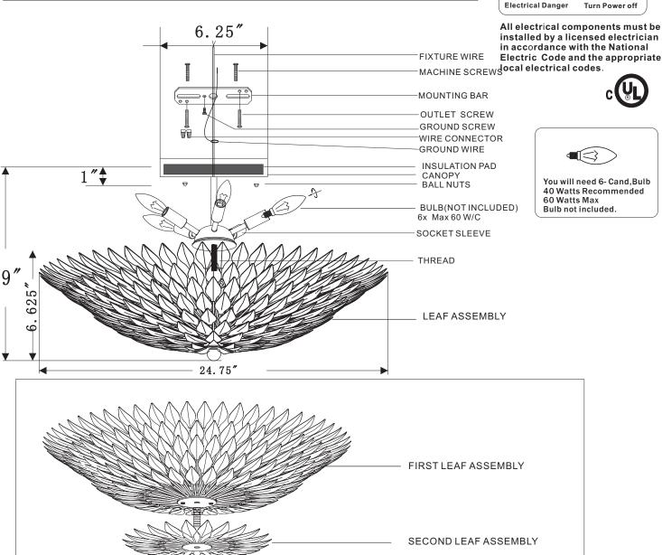
NOTICE: FOR REPLACING THE BULB, PLEASE UNSCREW THE LEAF ASSEMBLY AS SHOWN ABOVE
