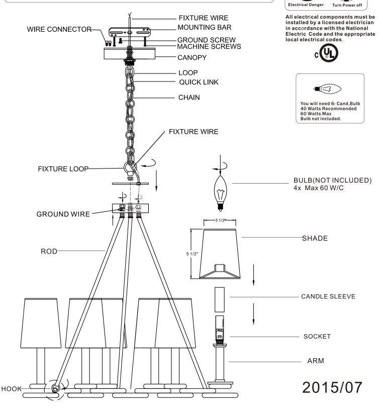
PS:After attaching the rod to hook on bottom frame, please pull the loose fixture wire only.(not the ground wire.)
