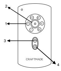
Fan **SPEED** buttons--1: Fan **OFF** button--2: **REVERSE** function button--3: **LIGHTING** button--4: Use to control ceiling fan speeds 1-6 Use to turn the fan off Use to control fan direction Use to control down-light and up-light (if applicable)
