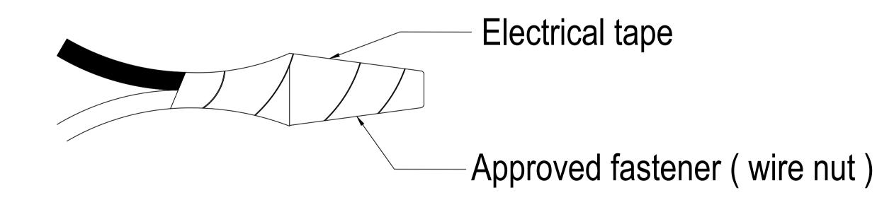
**7.** Connect the black fixture lead to the black wire in the outlet box. Fasten the joined wires as in step 6.
