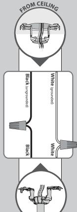
Using orange wire connectors from the  $\bigstar$  hardware bag, connect the black wire (ungrounded) from the ceiling to the black wire from the fan. Connect the white wire (grounded) from the ceiling to the white wire from the fan.
