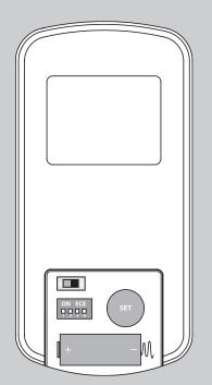
To change the battery, remove the battery door. Remove battery and replace with A23 or MN21 alkaline battery. Please observe proper polarity placement.
