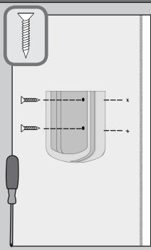
To install the transmitter cradle, hand-tighten the provided screws to mount the cradle to the wall.
