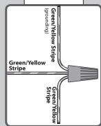
Using an orange wire connector from the hardware bag, connect the three grounding wires (green, green/yellow stripe, or bare copper) coming from the ceiling, downrod, and hanging bracket.
