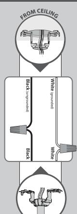
Using orange wire connectors from the hardware bag, connect the black wire (ungrounded) from the ceiling to the black wire from the fan.
