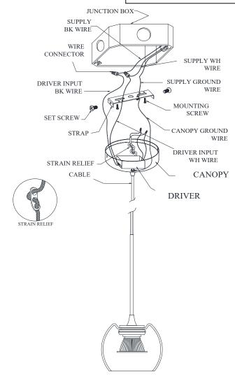
WARNING: DO NOT CUT THE PENDANTS CABLE. LOOP THE CABLE INSIDE THE CANOPY LIKE THE PICTURE SHOWS ON THE LEFT TO HAVE YOUR DESIRED LENGTH OF CABLE EXPOSING CANOPY.
