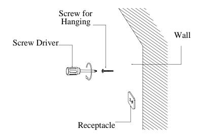
Rotate the hanging screw on the wall by screw driver.
