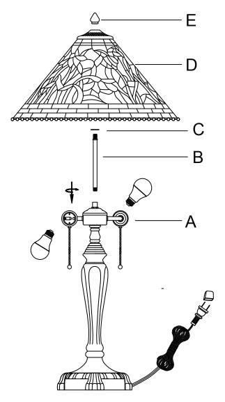
Use MAX 2 x 60 Wattage Type A bulb (bulb not included)
