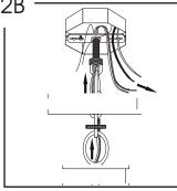
Slip screw collar ring and canopy onto chain, and hang fixture onto screw collar using an open link of chain. Close link. Thread wire and ground cable through screw collar ring, canopy, chain, screw collar, and through threaded tube on crossbar assembly. Pull wires through.
