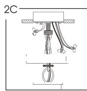
Strip 3/4" of insulation from wire ends. Connect house ground wire to fixture ground wire. Twist wires together using wire nut. Connect the black house wire to the smooth or black fixture wire. Twist wires together using wire nut. Connect the white house wire to the ribbed or white fixture wire. Twist wires together using wire nut.
