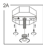
Screw crossbar assembly into junction box using outlet box screws. Thread screw collar onto threads of crossbar assembly.
