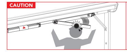
The awning arms contain tensioned cables. Always use caution, securely tie the awnings arms to the awning when performing installation, adjustments, or repairs. Sudden movement of tension arms can result in serious personal injury, product and/or property damage.
