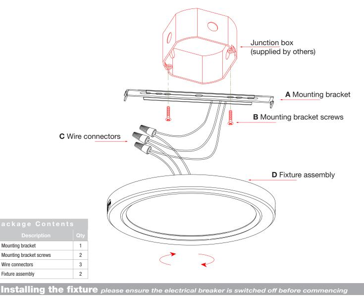
Attach the supplied Mounting bracket (A) to the Junction-Box. And secure in place with the two supplied Mounting bracket screws (B).
