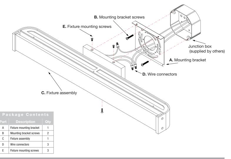
**Installing the fixture** please ensure the electrical breaker is switched off before commencing
